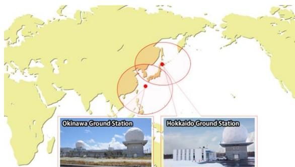
Also, communication periods between satellite and ground station are limited to when a satellite passes over the ground station. Therefore, it is necessary to establish network communication opportunities with multiple ground stations around the world.
